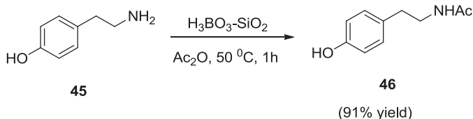
Scheme 19 Boric acid-catalysed acetylation of amine
