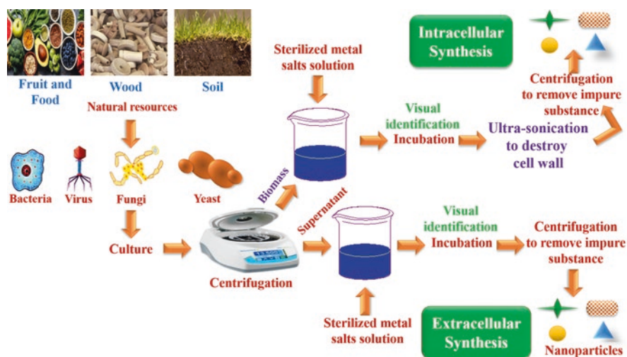
Fig. 6 Schematic presentation of a generalized protocol for green synthesis of nanoparticles by different microorganisms
